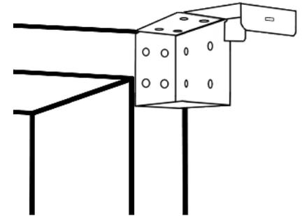
Mount center support brackets (if needed), near the center of the window. (Fig 3) Be sure to mount the support bracket (s) in positions that will not interfere with the operating mechanisms of the blind.
